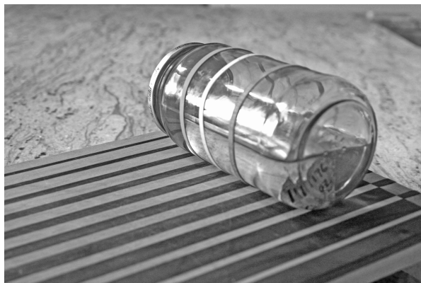
Figure 5 One can make a transparent snail ball using a jar, some corn syrup, and a moderately heavy metal cylinder.
