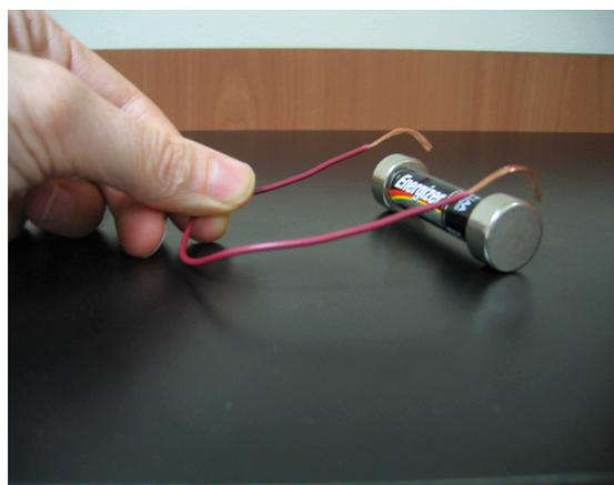
Figure 3: Construction used for a simple homopolar motor of the rolling type.
