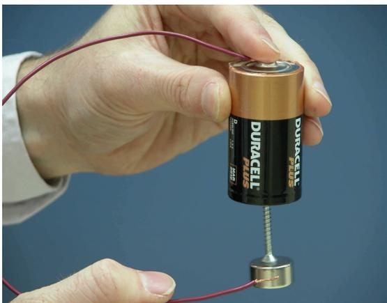
Figure 1: Construction used for a simple homopolar motor of the dangling type.
